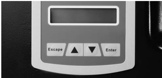
Figure 27. Nexus Display and Navigation Buttons
