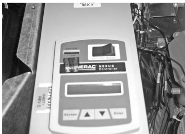
Figure 183. Remove 7.5 Amp Fuse
